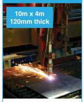
Flame cutting is ideal for cutting carbon steel and most metal alloys where cutting edge precision is not critical, or post machining is required.
