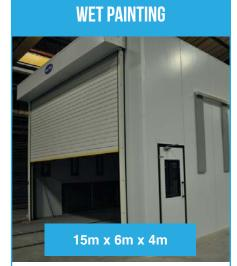
Our new 15m x 6m x 4m wet painting facility enables us to provide cost effective finishing solutions for large parts & assemblies. Working in-line with our shot blasting facility, it enables us to greatlty reduce waste and lead times.
